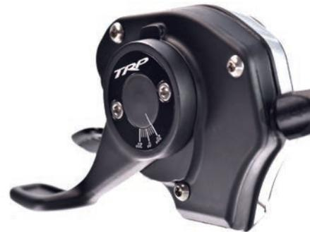
**Shifter:** Ergonomics are key to Aaron and he wanted something different for a reason. In addition to adjustability, TRP engineers looked at the cable release lever's ergonomics and devised a system to move it in a linear path to mimic the motion of a rider's thumb rather than rotating away.
